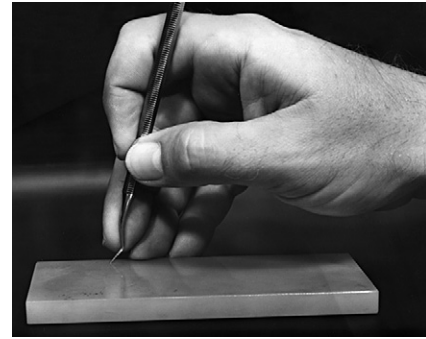
Online Fig. 23-2 Sharpening an instrument. Maintaining the proper angle of bevel and angle of the cutting edge to the stone is aided by resting the fingertips on the stone.
